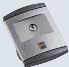
Key switch For 1 function, in a recessed version (shown) and surface- mounted version, including 3 keys. Operation of the automatic wicket door function is possible with an optional second microswitch.
